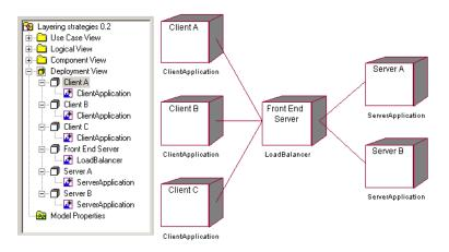
Figure 9: Deployment Model Describing Physical Distribution of Responsibilities
