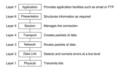
Figure 1: OSI 7-Layer Model (Responsibility-based Layering)
